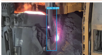
Crane hook tracking
